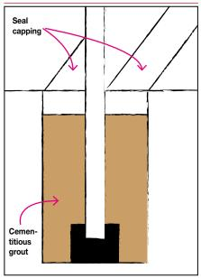
Use a ready-to-use anti-shrinkage mortar for injections and fixing in concrete.
